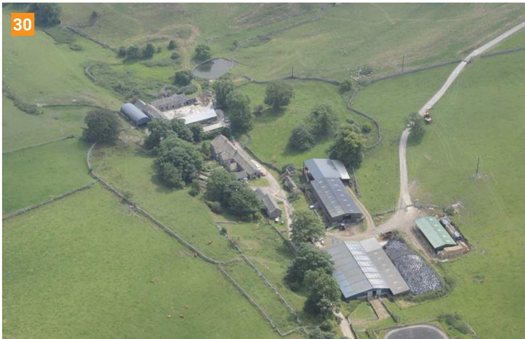
▲ 30. An example of a large Dispersed Multi-yard farmstead in Cales Dales, which developed at the meeting point of three routeways and is surrounded by paddocks with irregular boundaries. The buildings were all rebuilt in the early-mid 19th century, and comprise a Loose Courtyard in the background with cattle housing and a combination barn to all four sides, a Linear farmstead with a detached bakehouse at its far end and additional ranges of cattle housing along the main routeway passing through the site. This is a medieval farmstead site which developed from the grange farm of the Cistercian house of Roche Abbey. This type of development is echoed in many valleys in uplands of northern England.
