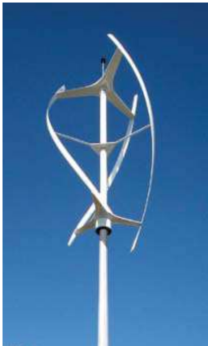
Figure 36. Vertical axis turbine (picture courtesy of Land Use Consultants)
