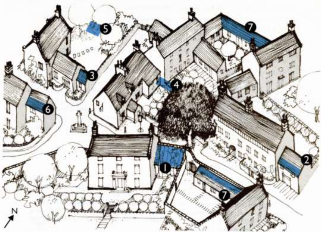
Figure 20. Illustrative guidance for locating solar technologies in a traditional village scene
