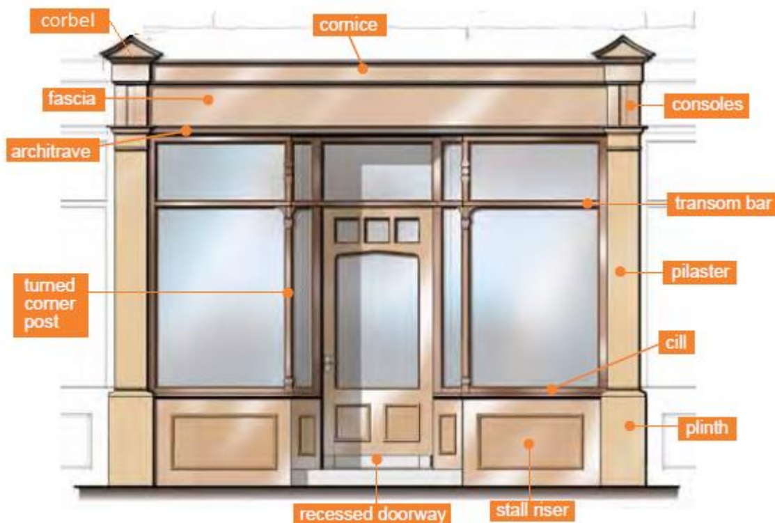
14. Main Components of a Traditional Shop Front
