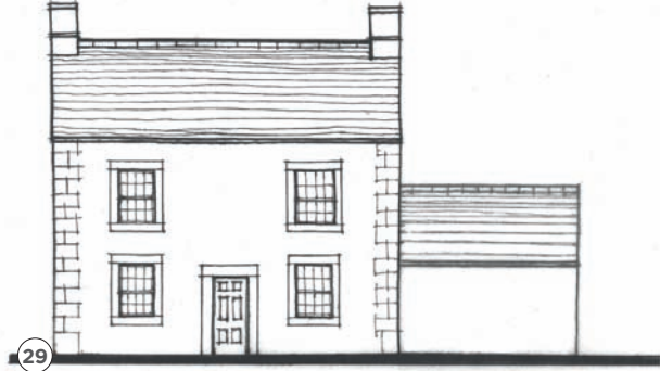
29: Although modest, the proportions of the single storey side extension to the right of the main building could be improved. The height to length ratios of the extension is different from that of the main building. The additional horizontality of the extension results in dis-harmony.
