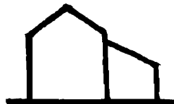
Lean-to roof at shallower pitch and stepped.
