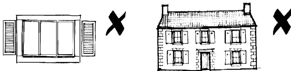
In both examples, the shutters clearly do not fit the windows.
