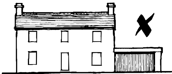
Prominent flat roof extension.
