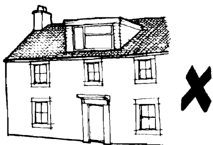
Large flat-roofed dormer dominates elevation.
